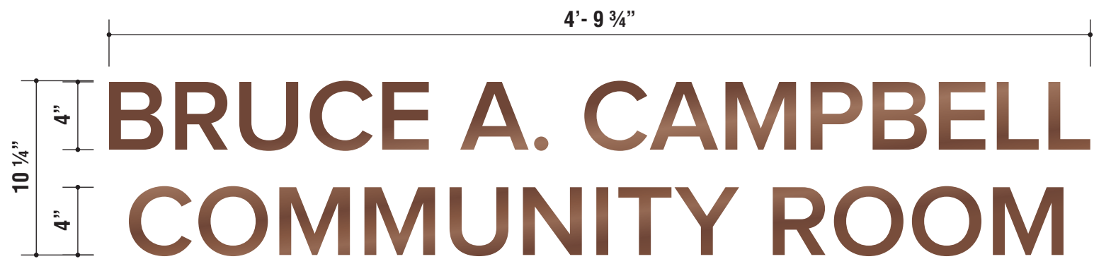
E Sign Elevation Layout Qty: (1) Scale: 1/8" = 1'-0" Manufacture and install 1/2" thick brushed medium bronze with black returns
